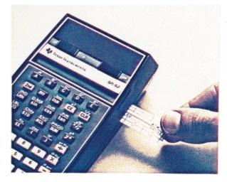
1. Insert card. Send the A-side of the prerecorded magnetic card through first.
