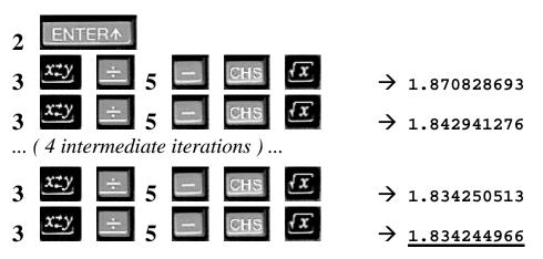
As the root is x = 1.834243184 we've got again about 7 *decimal places*, this time requiring just *eight* "mindless" iterations of the above **HP-35** sequence.
