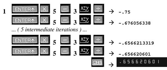
As the root is x = .6566204310 we've got about 7 *decimal places* by *routinely* performing just nine iterations of the above **HP-35** "program".
