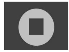
First of all, we need to write and enter a subprogram **CIRCLE** which will generate the required Z-map for this stereogram, assuming the darker area is the base plane (height=0), and the lighter circle-with-square-hole is above it, at height 1. The subprogram which will then fill **z**\$ with properly placed "0"s and "1" is:
